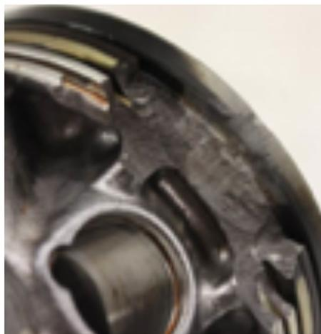
Two examples of piston damage due to LSPI (Source: [www.infineuminsight.com](http://www.infineuminsight.com))
